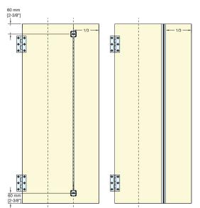
DOORS Measuring from the side of the door opposite to the hinges, install at 1/3 door width. Use One door straightener. For recessed and concealed straighteners install adjustor 60mm from top and bottom. Retrofit along whole length of door.
