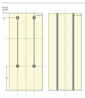
DOORS Recessed and concealed. straighteners do not need to travel down the whole length of a sliding door, only the top 3/3 of the door. Install at 1/4 and 3/4 door width Install 60mm from the top of the door. For Retrofit, install along whole length of door. Use 2 straighteners.
