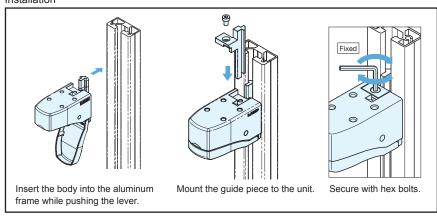
Can be installed to an aluminium frame that is already assembled. (see the instruction manual for details)
