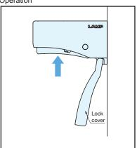
Open the cover and push the lever to move the unit up or down. The unit stops where the lever is released.
