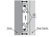
3 Hinge Installation After adjustments are finished, fasten fixing screws to complete installation. Please note: Vertical and depth adjustments will not be possible after this step.
