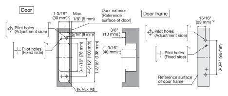
\*1 The diameter and depth of the pilot hole depends on the strength of the timber. Drill pilot holes before installing hinges. The position of the screw on the fixed side depends on the adjusted position of the hinge.
