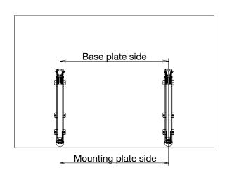
Ensure that the two LIN-X bodies are parellel by measuring both the base and mounting plate distances. 4 Connecting plate installation:
