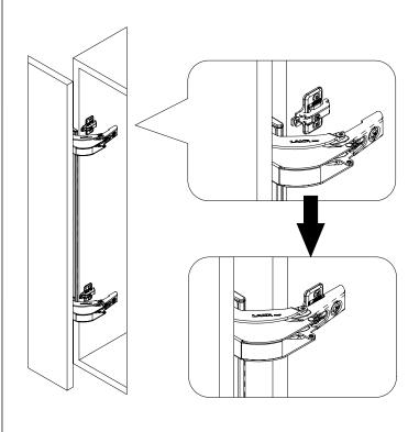
Ensure that the LIN-X body is securely attached to the mounting plates.
